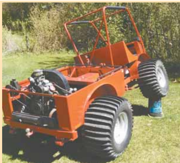
Riding on dune buggy tires, ATV oscillates and articulates at walking speed through rough terrain.
